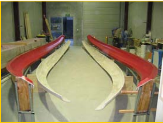
Deck parts released from molds.
