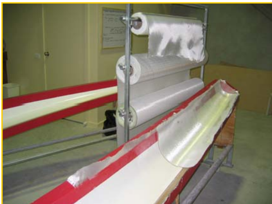
Decks being laminated.
