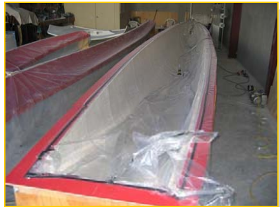
Vacuum-bagging the Balsa Core in.
